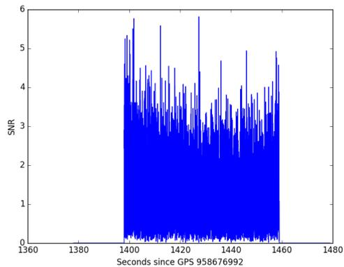
FIG. 2: A typical recovered SNR vs. Time graph from S6 run when the recovery has been considered successful
